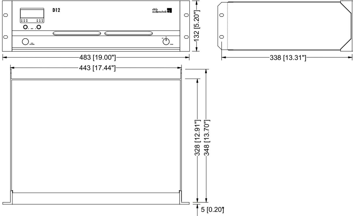
Fig. 25: D12 enclosure dimensions in mm [inch]
