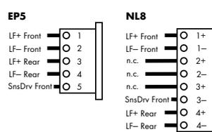
Tab. 7: Loudspeaker pin assignments and equivalents
