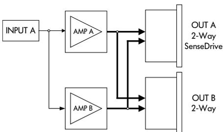
**Fig. 19: D12 Input/Output routing 2-Way Active mode with standard input routing**
