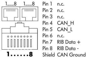
**Fig. 10: Pin assignment for remote control (RJ 45)**
