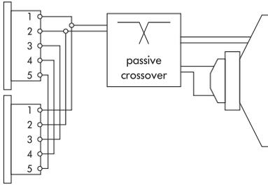
**Fig. 4: Connector wiring**
