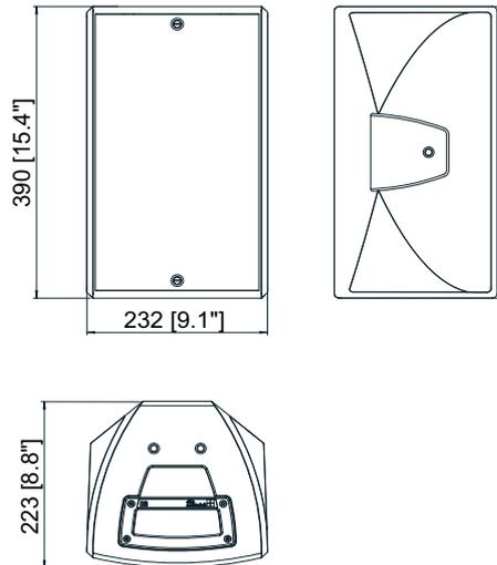
**Fig. 12: E8 cabinet dimensions in mm [inch]**
