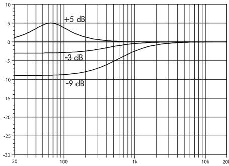
**Fig. 6: Frequency response correction of CPL circuit**
