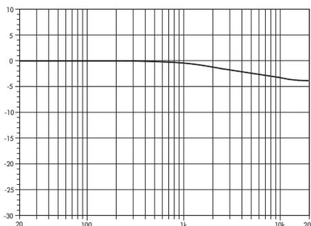
**Fig. 5: Frequency response correction of HFA circuit**
